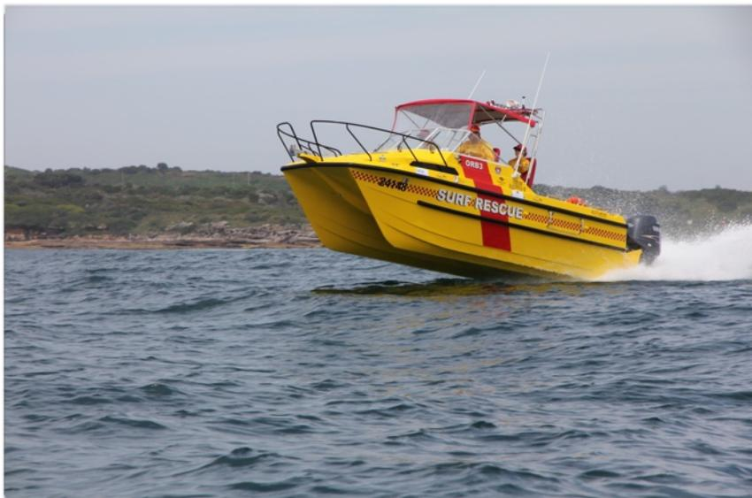
Stronger, lighter smarter, cleaner ... are all words which help describe our next generation rescue vessel. Our new Kevlacat, is hand laid with Kevlar (yep, that's the bullet proof material) giving the hull increased strength without added weight. It carries almost 200 litres more fuel and fresh water yet remarkably it tips the scales at less weight than our previous craft. The new Surf branding is something we should all be proud of when we see the craft patrolling off Randwick and
